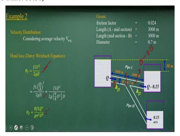
So we just substitutes to compute head loss because this amount is a Q amount of waters and this pipe will be Q minus 0.15 okay. So you will compute the head loss. That is what we have derived it and you compute this head loss components. Sometimes we write in terms of Q or you can write in terms of V, that is not a big issue.
