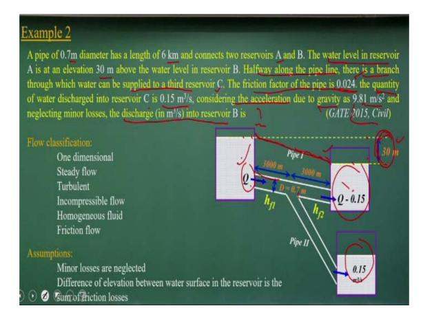
Now you take it the second problems which has the GATE 2015 problems is that the pipe of 0.7 meter diameter has a length of 6 kilometer connects the two reservoirs okay and the water level in the reservoirs is 30 meter above the water level of reservoir B okay. Halfway along this pipeline there is a branch. Water is supplied to the third reservoir C. Then friction factors of the pipe is given.
