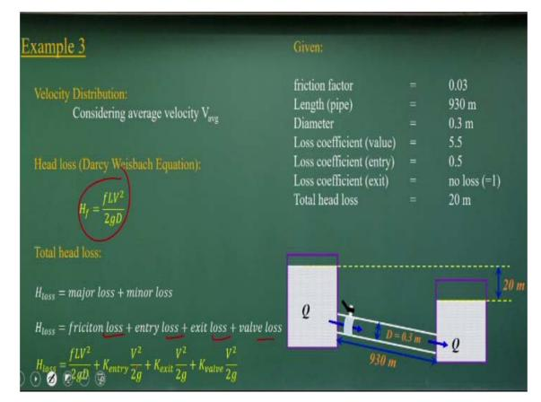
We will use this energy losses, frictions losses, entry losses, exit losses, valve losses, all components are there.
